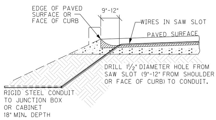
PIEZOELECTRIC SENSOR INSTALLATION
